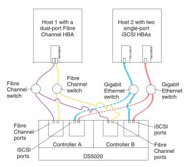
Figure 65. Example of a multiple-host, multiple-port, multiple-switch configuration
